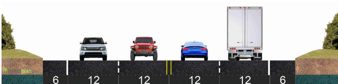
Figure 2-9 Alternative 4B – Conceptual Cross-Section
