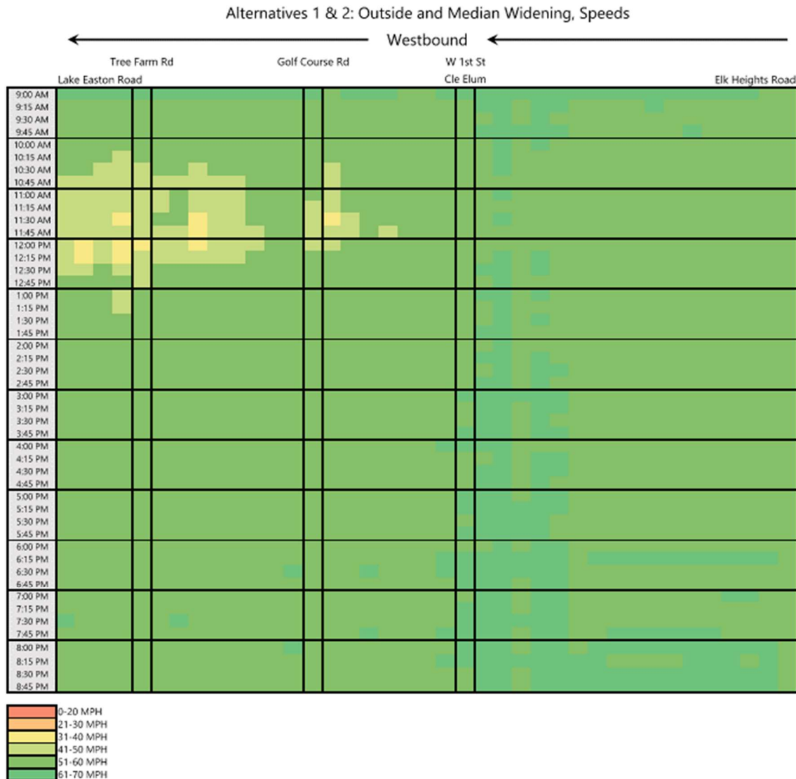
Figure 5: Alternatives 1 and 2 Modeled Travel Speeds by Time of Day and Location Along Corridor
