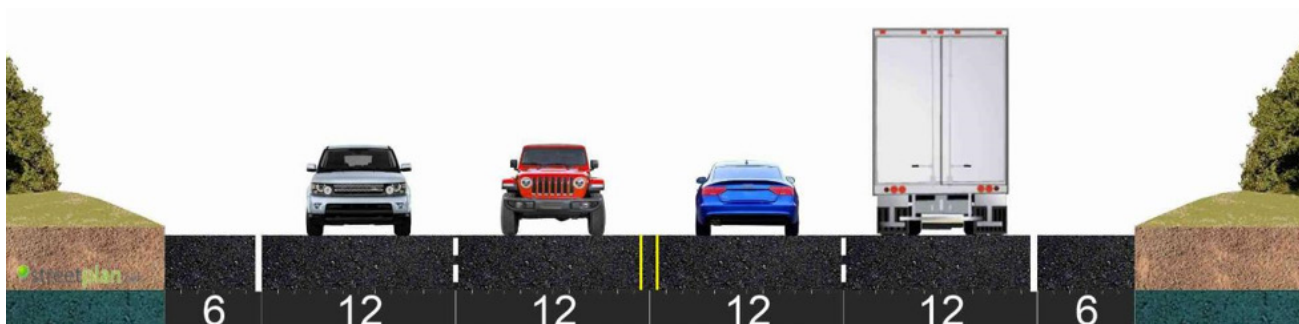
Figure 2-7 Alternative 4A – Conceptual Cross-Section
